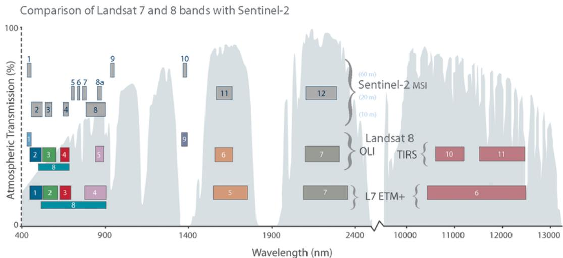
**Figure 4:** Graphical representation of the spectral bands of MSI/Sentinel-2A compared to the cameras of the Landsat 7 and 8 satellites. The axes depict the wavelength in nanometres ( $1 \text{ nm} = 10^{-3} \mu\text{m} = 10^{-9} \text{ m}$ ) and the terrestrial atmospheric transmission (grey) in percent (Credit: NASA, <https://landsat.gsfc.nasa.gov/sentinel-2a-launches-our-compliments-our-complements/>).
